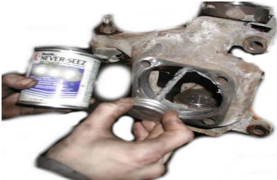
15. Install the spindle over the axle and install the 4 - 14mm Socket head cap bolts (Red thread locker recommended Tighten to 105 ft lbs. Make sure you install the dust shield before the spindle.
