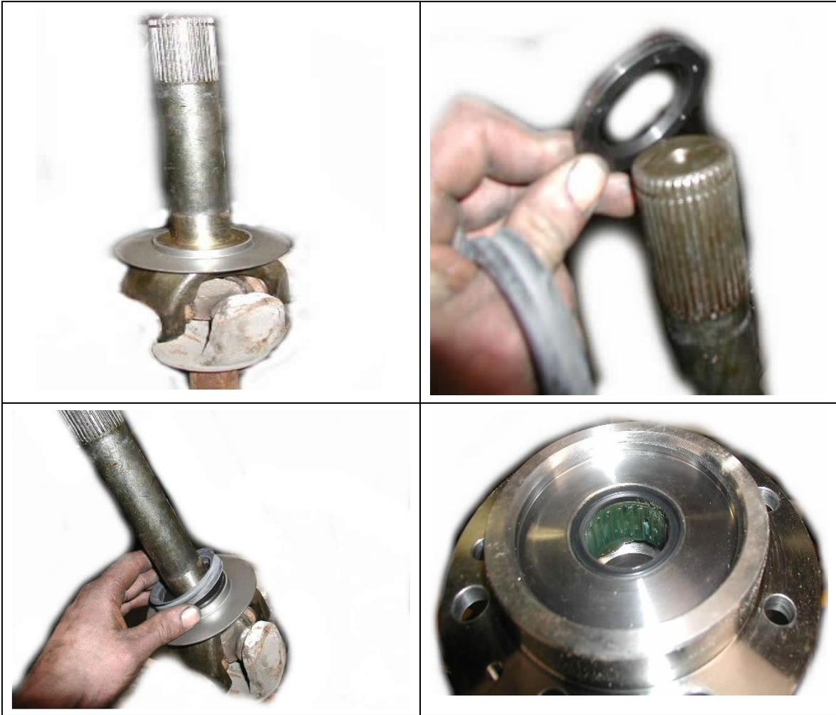
6. Install wheel bearings into new wheel hubs.
